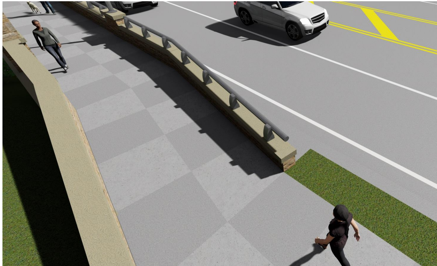
Interior Barrier End Section Taper
