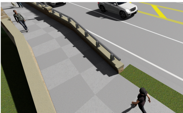
Interior Barrier End Section Taper
