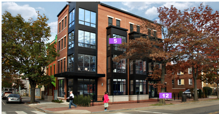
5 Use Balconies in mixed-use buildings to provide eyes on the street (5.C.1-B1) 12 Avoid large setbacks unless used for public benefit—like outdoor seating, landscaping, or plazas (5.C.1-D2)
