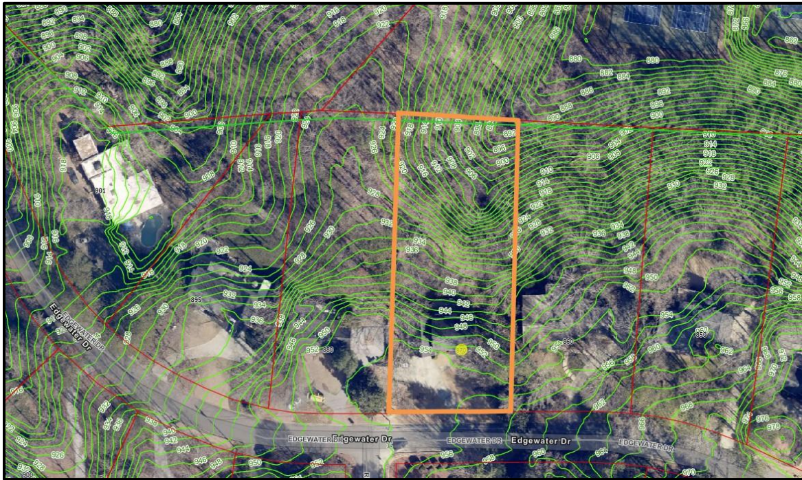
Aerial view showing topography lines (in green) of subject property and surrounding parcels
