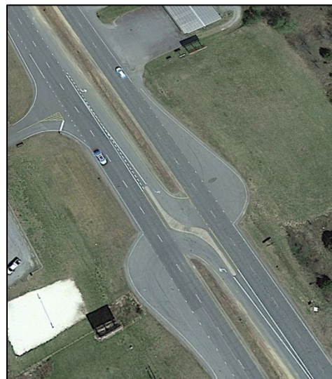
Figure 12. Truck/Emergency Vehicle U-Turn Accommodation (US 74, Whittier, NC)
