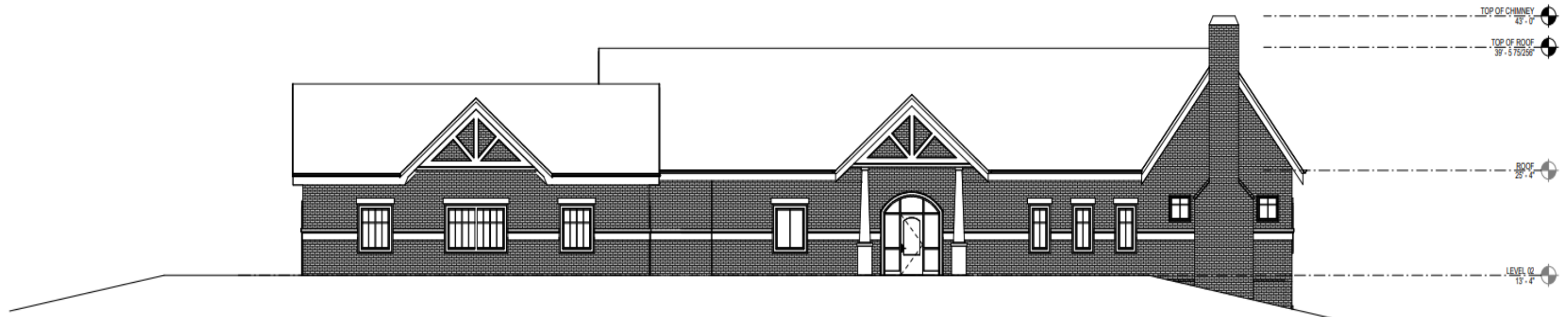
2 BUILDING ELEVATION - NORTH 1/8" = 1'-0"
